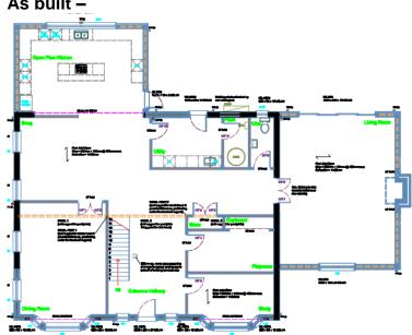
The rear extension remains 4.5 metres in depth but has been brought in line with the side wall of the house rather than inset. The previously approved lantern roof has been removed and now has a flat roof.
