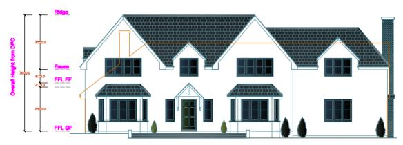
6.7 The elevation drawings of the approved plans show a height of the extended property with a ridge height of some 7.1 metres taken from damp proof course (DPC).
